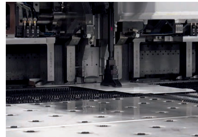
Synthesis steel frame panel being made to exact specification on the state-of-the-art bending machine
